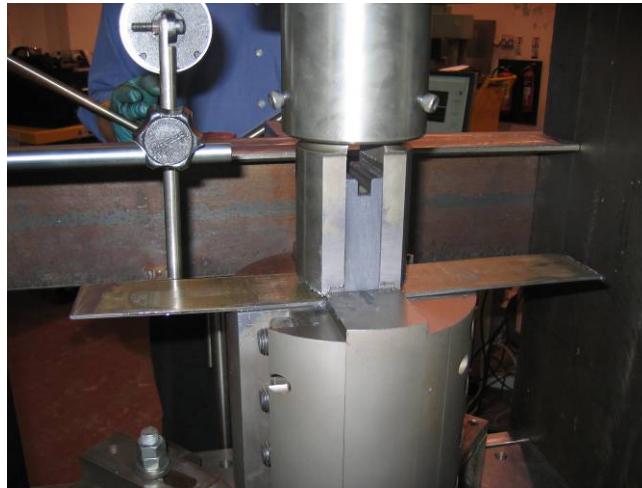
Figure 2.7: Tool design for I-ECAP of sheets
