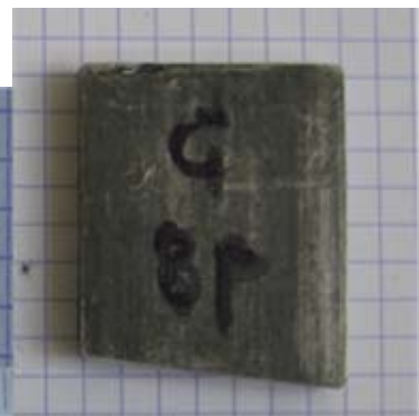
Figure 3.3: Material flow at the tail of a rectangular sample (left) and resulting surface marking (center); the “usable part” of the sample (right) is about 35 mm x 40 mm
