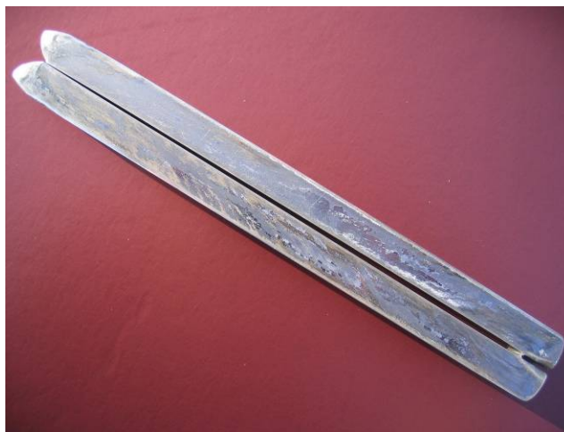
Figure A.6.4: ECAP processed bars
