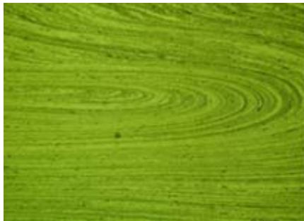
Figure 3.3: Material flow at the tail of a rectangular sample (left) and resulting surface marking (center); the “usable part” of the sample (right) is about 35 mm x 40 mm
