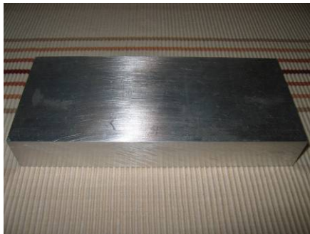
Figure A.6.2: Block of AlMgSc
