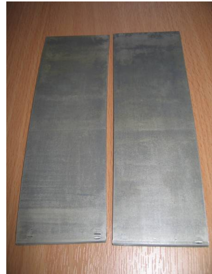
Figure A.4.2: I-ECAP'ed strips
