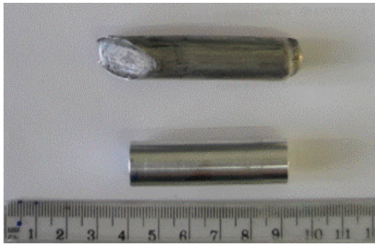
Figure 3.2: Cylindrical and rectangular ECAP sample after several ECAP passes
