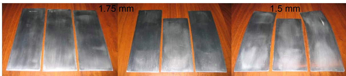
Figure A.4.3: Strips after 6 passes of I-ECAP and machining with sand paper
