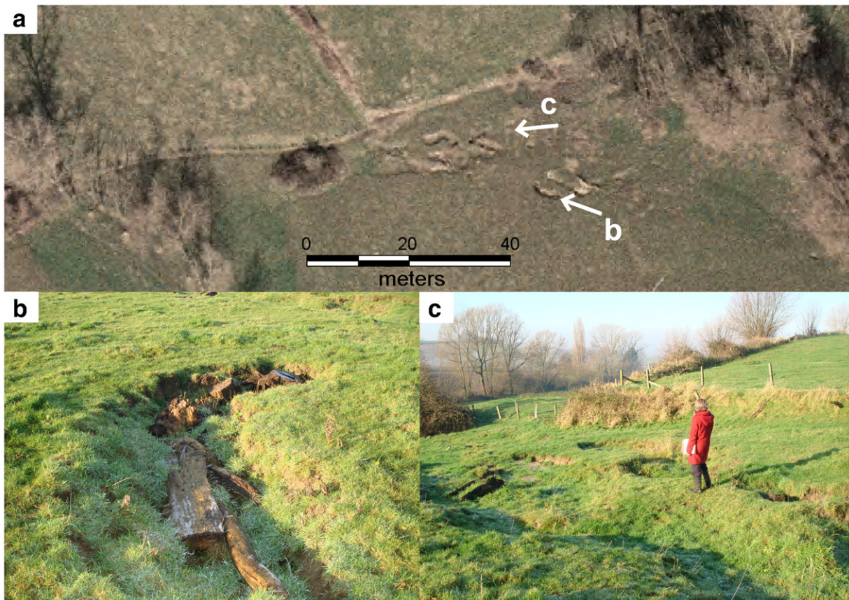
Fig. 2. Photographs of the study area. (a) Aerial orthophoto with indications of possible collapsed pipes. (b and c) Terrestrial photos of the sites with collapsed pipes (Kluisbergen, December 2007; see (a) for location).
