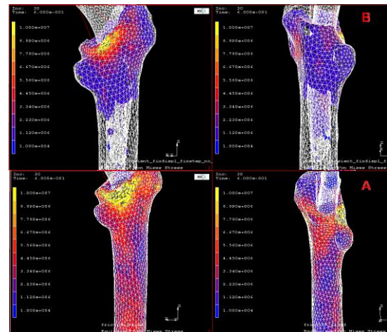
Figure 5: Von Mises stress distribution at an intermediary step of insertion (colored zones) (A – frictionless contact and B – contact with friction)
