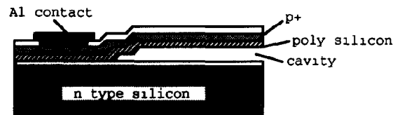
Fig 9 Principle of a surface micromachined pressure sensor by etching the oxide from underneath the polysilicon, a cavity can be created. The doped p + region is used as the movable electrode for the sensor
