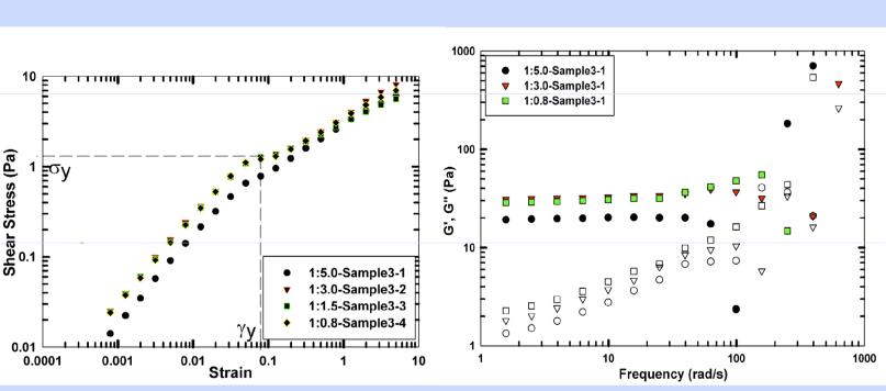
Oscillatory measurements show a strong elastic behavior in a wide range of strains and frequencies, up to a strain of 0.1 at which the emulsion begins to yield. The yield stress value of ~1 Pa is in excellent agreement with the plateau value of the steady shear stress.
