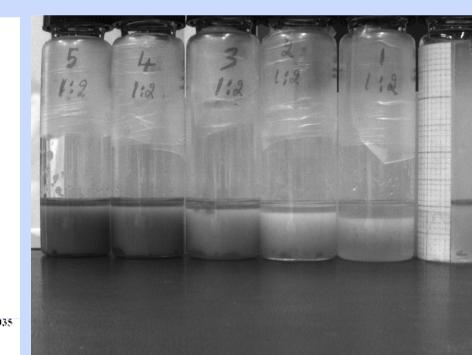
All emulsions show an excellent stability over time (> 6 months). The efficiency in emulsion formation is high even at very low FGS concentrations (E-3 wt%/vol). The emulsification power increases with FGS content and water fraction up to a constant volume fraction of <u>0.85</u> (emulsion:total volume).
