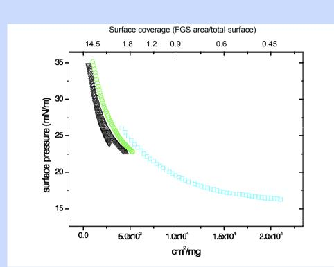
FGS at water-air interface Pressure-Area isotherms at different surface coverage
