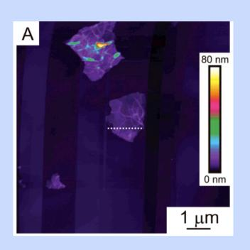
Mean thickness 1.7 nm Surface area  $600-900 \text{ m}^2/\text{g}$  (BETNitrogen) 1850 m²/g (MB dye Ethanol Suspension) MJ McAllister, Chem. Mater. 2007, 19, 4396-4404
