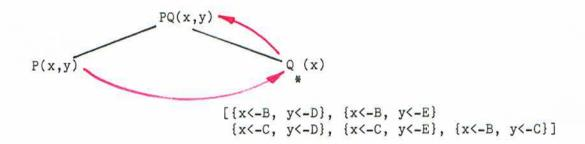
$Q_{*}$  does not change its (empty) set of untried procedures. Instead of deriving the current solution set for PQ, the additional dependency has forced us to first derive a current solution set for Q(x), P(x,y). The further reduction to derive all solutions for the initial goal statement can be done usual.
