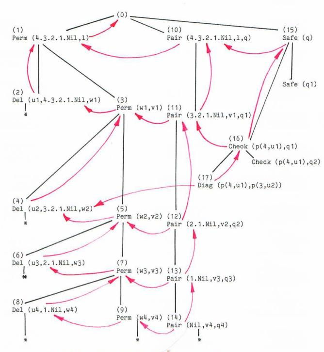
And-tree and dependecy-graph at the point where call (17) causes a failure.
