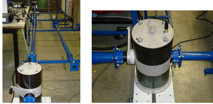
Figure 2: Picture of the flow-acoustics test rig (left) and an in-line loudspeaker (right).
