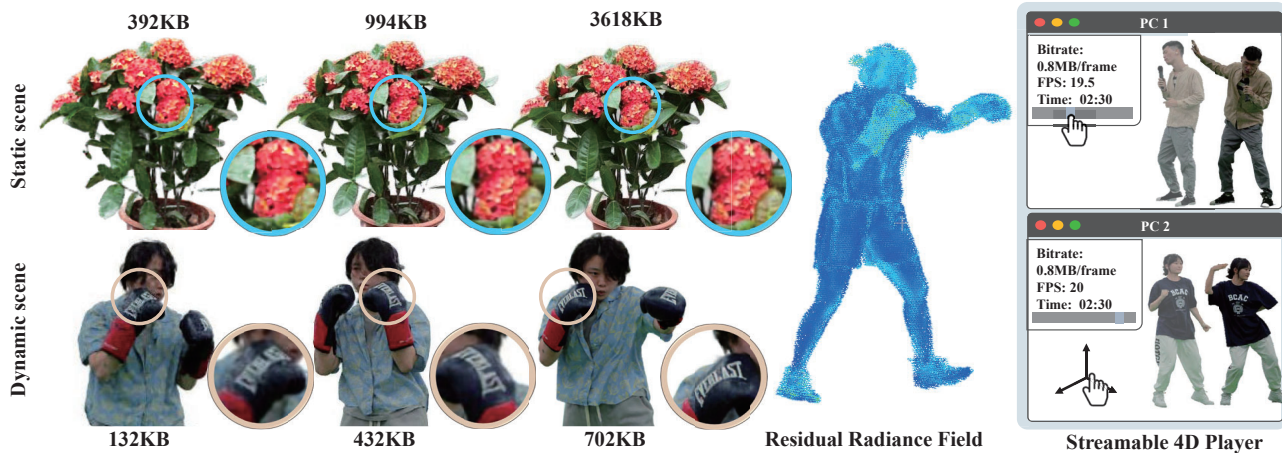
Figure 1. Our proposed ReRF utilizes a residual radiance field and a global MLP to enable highly compressible and streamable radiance field modeling. Our ReRF-based codec scheme and streaming player gives users a rich interactive experience.
