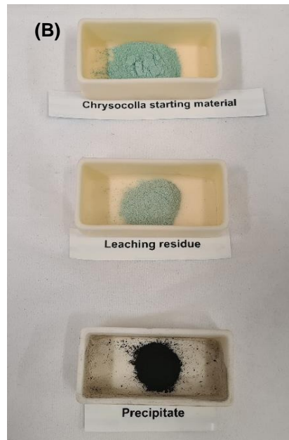
Figure 9. (A) Upscaling of leaching in a 1 L reactor and (B) overview of the different samples: chrysocolla starting material, leach residue, and copper sulfide precipitate.
