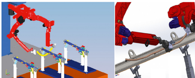
Fig. 5. Automated dual arm cabling assembly: collision detection during manipulation [157].
