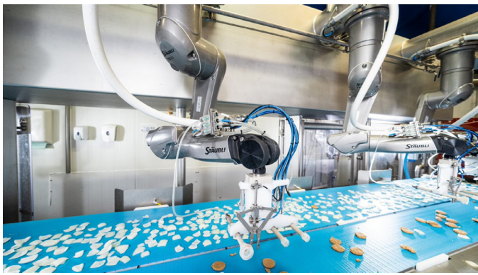
Fig. 10. Fully automated meat skewering machine [218].
