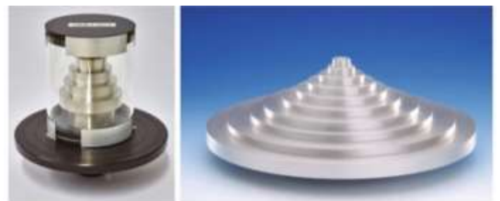
Fig. 29. Step cylinders: (left) standard of NMII, Japan with 50 mm max diameter and central bore hole [28]; (right) 250 mm standard of PTB without central bore hole ([21],[28]).
