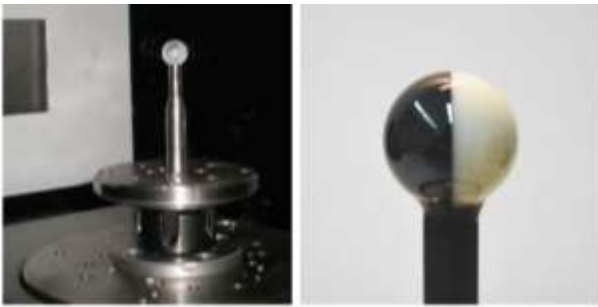
Fig. 27. Werth@ universal calibration sphere (left, [67]) and multi-material sphere developed by PTB (right) for testing XCT systems.
