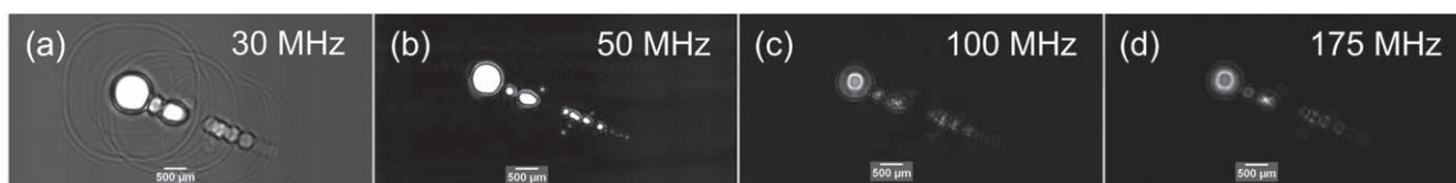
Figure 5. SAM images on the void induced by the 25 \mu\text{m} polymer particle scanned by different transducers: (a) 30 MHz, (b) 50 MHz, (c) 100 MHz, and (d) 175 MHz under 775 \mu\text{m} full-thickness top Si. The void residue behind the particle are observed. The gain parameter was tuned to obtain the clear quality for 30 MHz, 50 MHz, 100 MHz, and 175 MHz as 10, 10, 20, and 20, respectively.
