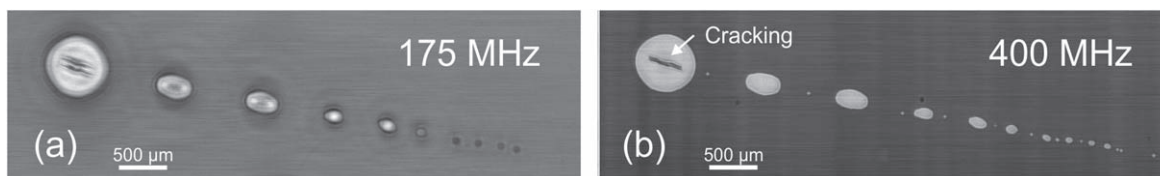
Figure 6. SAM images of the void induced by the 25 \mu\text{m} polymer particle under the 50 \mu\text{m} top Si scanned by (a) 175 MHz and (b) 400 MHz transducers. The gain parameter under the 50 \mu\text{m} for 175 MHz and 400 MHz transducer are 20 and 40.
