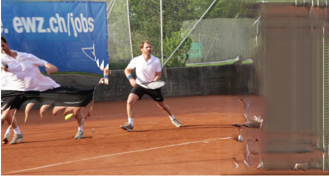
Figure 4. Video inpainting method from Gao et al. [7] applied to video outpainting. The center of the image was used as input, the left and right sides are completed.
