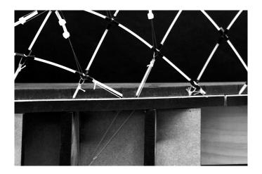
Figure 17: The supports in the physical model consist of a small socket and a tension cable running through the support plate.
