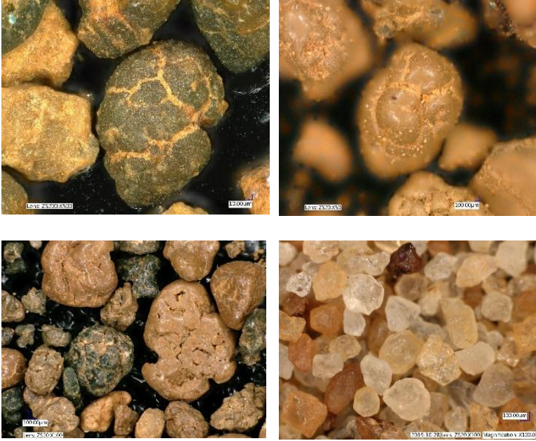
Fig. S1. Light microscopy images of glauconite fraction of GS from Lubbeek. Glauconite pellets showing signs of strong oxidation, with Fe (oxy)hydroxides coating on the glauconite, as well as on the quartz grains (right in the 2 nd row).
