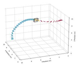
Fig. 2: Solution of the one rectangular gate problem, with the approach stage, fly-through stage and fly-away stage highlighted in red, yellow and blue respectively.
