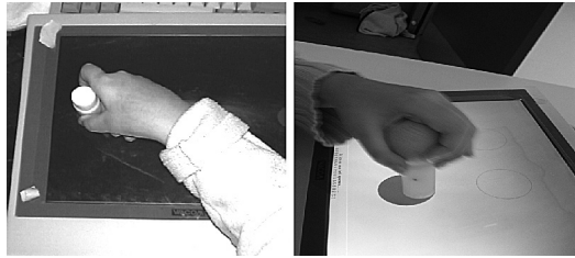
Figure 1. The experimental set up with a digitizer as colour LCD monitor. The tablet is placed horizontally directly in front of the participant. Adaptations in equipment have been made if disablement was too severe to hold the puppet.
