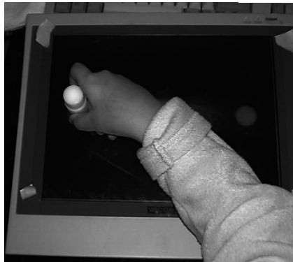
Figure 1. The experimental set up with a digitizer as color LCD monitor. The tablet is placed directly in front of the participant. The digital pen is embedded in a "puppet" of 2.5 cm by 7 cm.
