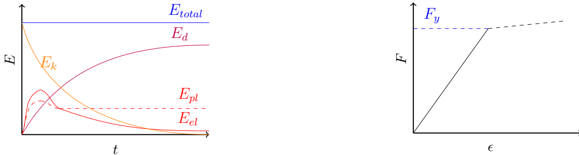
(a) Energy balance of one simulation where all the kinetic energy E_k is transformed into deformation energy E_d , and energy in the springs E_s ; (b) Illustration of the stress-strain behaviour of different material models. Note that a little energy is lost in hourglass modes E_h , while the total energy remains constant
