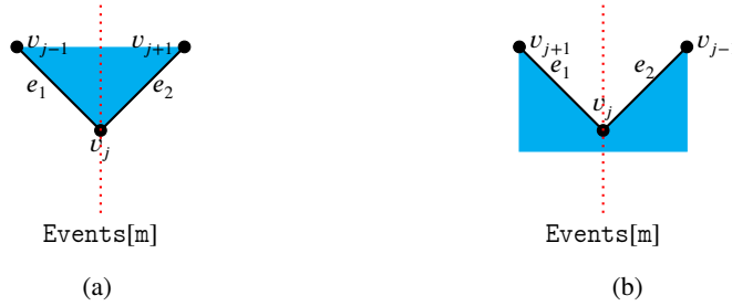
Figure 13: Updating ActiveEdges: case b: Events[m] is the x-coordinate of the right endpoint of edge e_1 and the left endpoint of edge e_2 . Information of edge e_1 is removed and information of edge e_2 is added to ActiveEdges.
