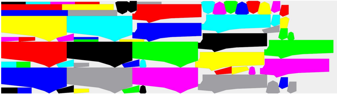
Figure 18: Placement result for data set 'Trousers' semi-discretized with R = 0.2 and 2 allowed rotations ( \Delta\theta = 180^\circ ). Resulting strip length = 283.6.
