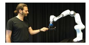
Fig. 1. Example of a handover between human and robot of a small cylindrical object.
