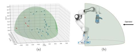
**Fig. 6.** (a) Successful (blue) and failed (red) attempts at handovers, drawn within the workspace of the robot (green). Each short line piece indicates the object orientation when starting the transfer. (b) The same workspace shown with respect to the robot.
