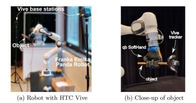
Fig. 5. Overview of the experimental setup. A Franka Emika Panda robot holds an object using a qb Softhand. The object consists of a cylindrical rod with an HTC Vive tracker mounted on top. The position and orientation of this tracker is measured by two static HTC Vive base stations placed on tripods.
