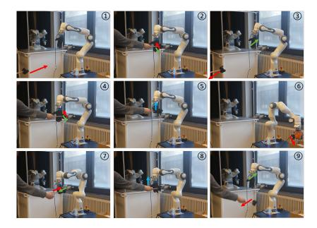
**Fig. 7.** Overview of different phases during a practical bidirectional handover. The human's motion is indicated with red arrows, the robot's motion with green arrows and the estimated contact force direction in blue. For the human-to-robot handover, (1) - (4) corresponds to the *reaching phase*, (5) is the *passing phase* and (6) is the *retraction phase*. (7) - (9) is the robot-to-human handover.
