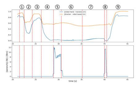
Fig. 8. Position and force evolution during a bidirectional handover. Top: distance between robot hand position and object position (orange) and distance between robot base and object (blue). Bottom: norm of the filtered contact force (blue).
