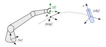
Fig. 3. Trajectory following towards object transfer point during reaching phase.
