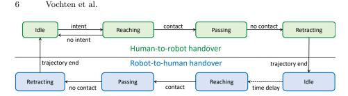
Fig. 2. Visualization of phases and transitions for a bidirectional handover.
