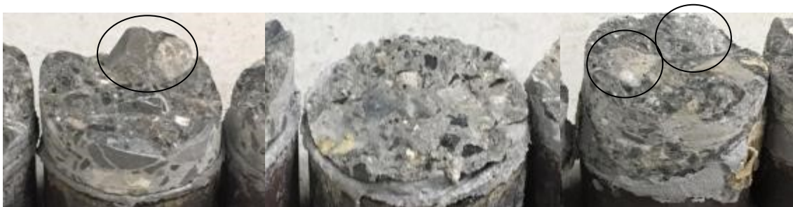
Figure 8. Example of failure modes of unprepared-CC (left) JH-CC (middle) and WJ-CC (right) substrates under STS testing. The encircled zones show failures at the interfacial transition zone (ITZ).
