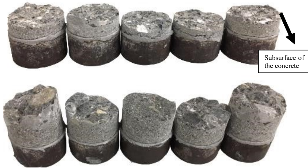
Figure 10. Bond strength failure modes of unprepared-CC (top) JH-CC (middle) and WJ-CC (bottom) samples at 28 days.
