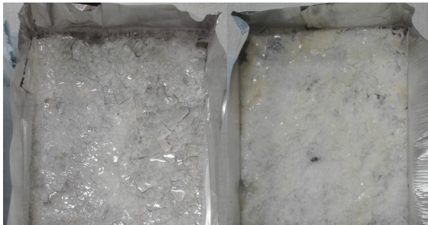
Figure 1. The plan view of dry silica gel layer for samples treated with CNS (left) and the combined application (right).
