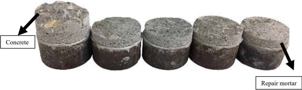
Figure 9. Bond strengths results. Error bars represent the standard error. Means with the same letter indication are not significantly different.
