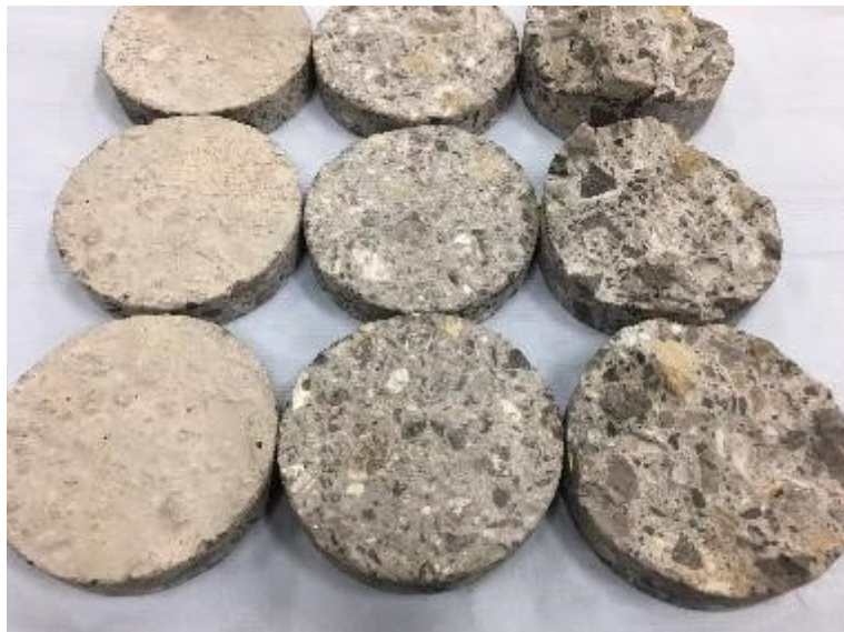
Figure 2. Prepared thin samples of CC for vacuum absorption test.
