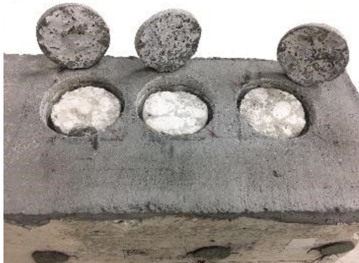
Figure 16. Pour-applied bacterial treatment - failure while drilling cores.
