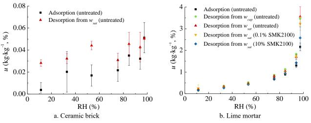
Fig. 4 The sorption isotherms obtained from the desiccator tests
