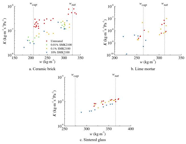
Fig. 7 The liquid permeabilities obtained from the falling-head water column tests.
