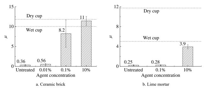
Fig. 9 The equivalent moisture transport resistance factors obtained from the drying tests
