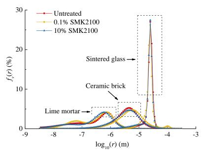
Fig. 3 The pore volume distribution obtained from the mercury intrusion tests
