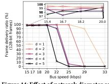
Figure 14: Effect of network diameter on reliability.
