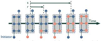
Figure 4: Changes between symbols propagate through the network in a wave-like fashion.
