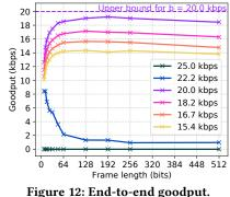
Reliability primarily depends on frame length and favours short frames: delivery ratios decrease by roughly one percentage point when using 128-bit instead of 32-bit frames. Contention, on the other hand, has no significant effect. When configuring two nodes to reply to a request using a different priority code, the high-priority frame is received as reliably as frames that are not contended with.
