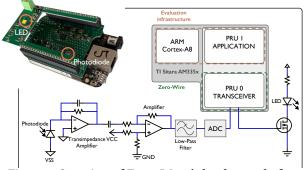
Figure 7: Overview of ZERO-WIRE's hardware platform.
