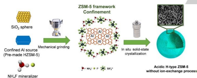
Figure 10. Proposed reaction mechanism for the creation of a hollow sphere with stacked ZSM-5 zeolites. [185] Reproduced with permission of Wiley-VCH Verlag GmbH & Co. KGaA.
