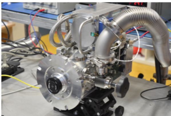
Fig. 1. Left. Picture of the MIRC-X C-RED ONE. Right. Scheme of the experimental setup. 1: H band single-mode fiber fed by a white-light source; 2: Dispersion prism; 3: Camera cold stop and baffle; 4: Low pass cold filter; 5: Detector.
