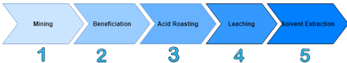
292 293 Figure 1. Processing steps of REEs from mining up to solvent extraction. 1) Mining of 294 REE from host material 2) Physical removal from host material 3) Decomposition of 295 beneficiated ores (sometimes referred to as cracking) 4) Transformation into a REE 296 chlorides 5) Separation of individual REOs 297 298
