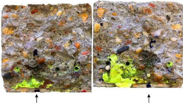
Fig. 11. Crack surfaces (60 x 60 mm 2 ) of one of the best performing CAPS specimen of lab 1. The hardened PU can be seen as fluorescent yellow. Arrows indicate the capsule from which fresh PU (visible as a dark stain) leaked on the surface when the specimen was broken. Image is highly saturated to improve visibility.
