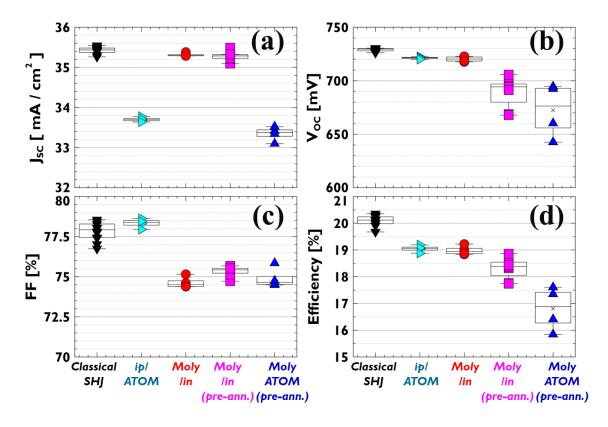
Figure 10. Performance comparison between classical SHJ, partial-doping free (Moly/in) and fully doping-free cells (MolyATOM). (a)  $J_{SC}$ , (b)  $V_{OC}$ , (c) FF and (d) efficiency. ip/ATOM data is from [41].
