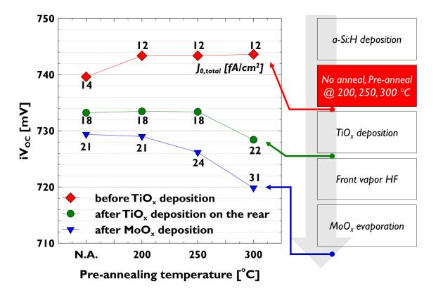
Figure 6. Progress in iVoc of pre-annealed or not-annealed samples at different process steps. The numbers in the figure are the  $J_{0,total}$  values of samples based on a  $J_{SC}$  of 36 mA/cm<sup>2</sup>.
