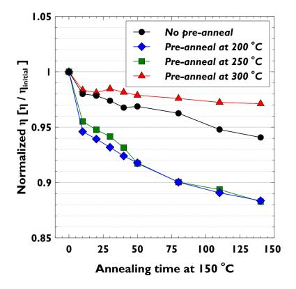
4.2. Dependence of thermal stability on pre-annealing temperature at cell level
