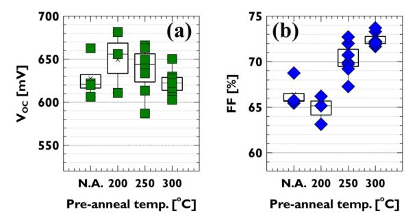
Figure 7. (a)  $V_{OC}$  and (b) FF of MolyATOM cells as a function of pre-TiO<sub>x</sub> annealing temperature.
