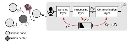
Figure 1: A WASN containing a fusion center along with multiple sensor nodes. Each sensor node is represented in three basic layers along with their energy consumption, i.e. sensing, processing and communication layer with  $\mathcal{E}_S$ ,  $\mathcal{E}_P$  and  $\mathcal{E}_T + \mathcal{E}_R$  respectively. [49]
