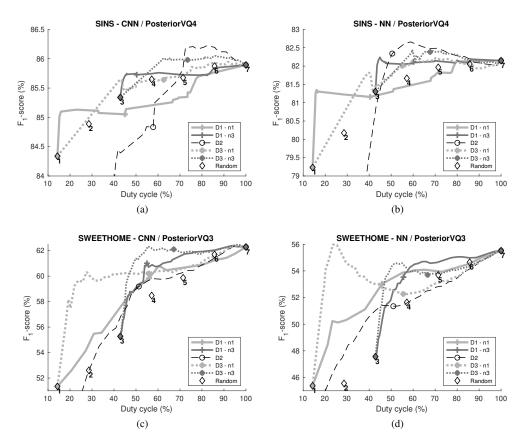
Figure 11:  $F_1$ -score with respect to the duty cycle of a sensor node for PosteriorVQ fusion at a precision of 4/3 bits for SINS and SWEET-HOME dataset respectively. Various dynamic sensor activation strategies are shown with respect to the threshold  $\rho$  along with random selection of sensor nodes.
