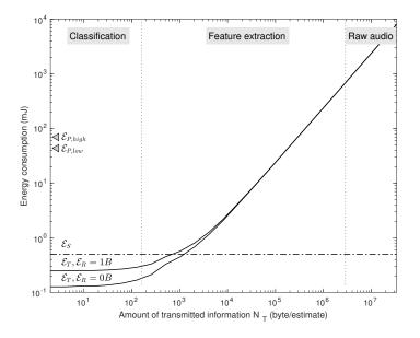
Figure 2: Energy consumption of each layer in a WASN in function of the amount of communicated bytes.<sup>1</sup>
