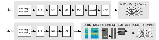
Figure 4: The classifier architectures ranging from low to higher computational complexity: NN and CNN.
