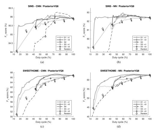
Figure 10:  $F_1$ -score with respect to the duty cycle of a sensor node for PosteriorVQ fusion at a precision of 8 bits. Various dynamic sensor activation strategies are shown with respect to the threshold  $\rho$  along with random selection of sensor nodes.
