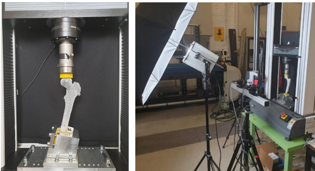
Fig. 4: Images of the experimental setup. The distal part of the femur is fixed onto the test machine with a holder that positions the femur such that its shaft is under an angle of 12° with respect to the loading axis (left). Two cameras and a cold light source are positioned in front of the test device for DIC recording (right).
