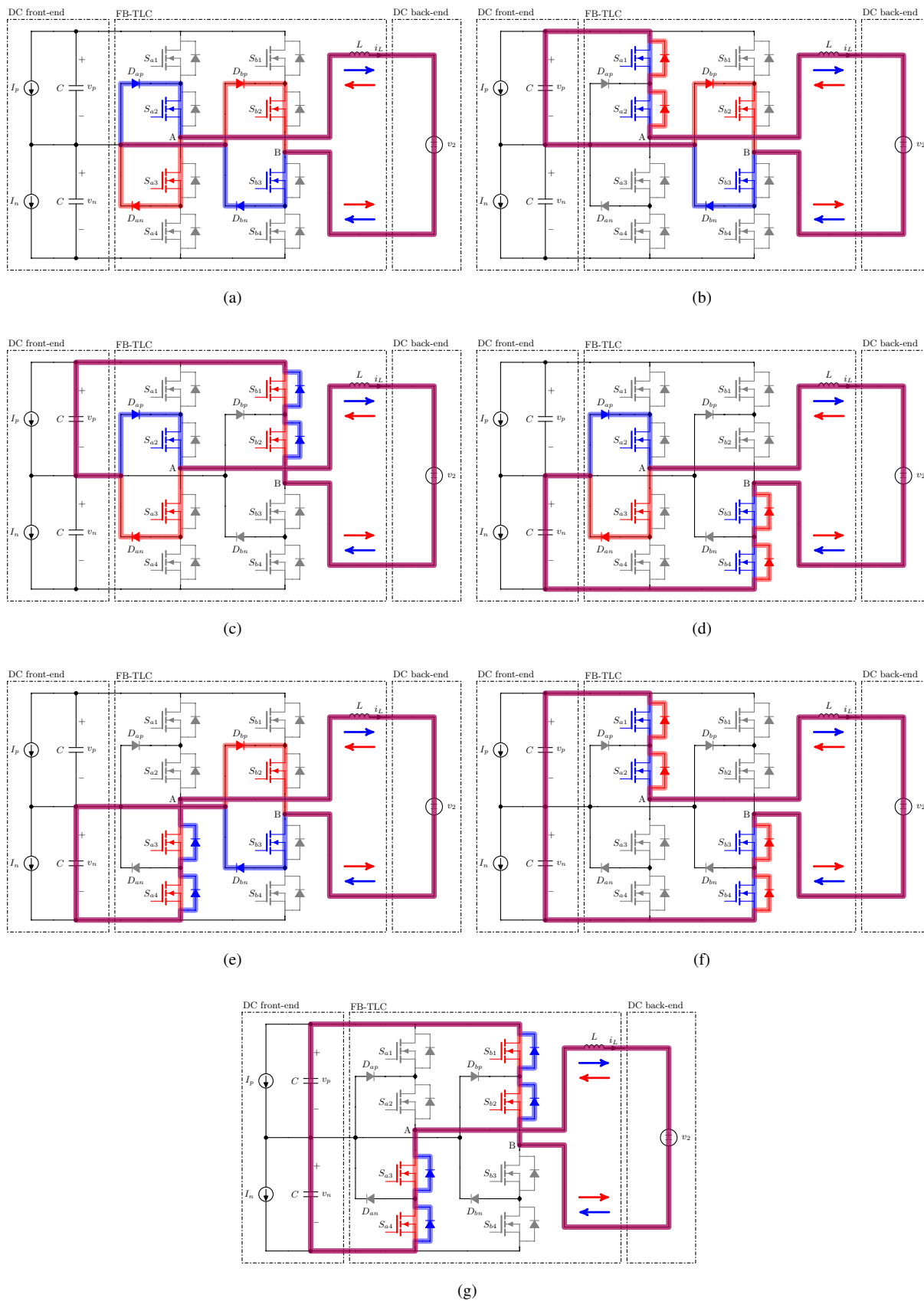
Fig. 2: Conversion stages of the FB-TLC (red: i_L < 0 , blue: i_L > 0 )
