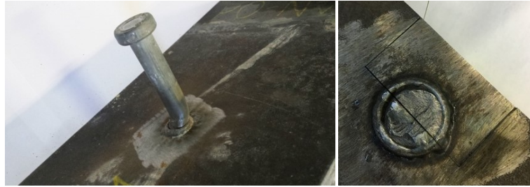
Figure 18: Plastic deformation of the stud (left) and cutting the sample using a wire-EDM (right)
