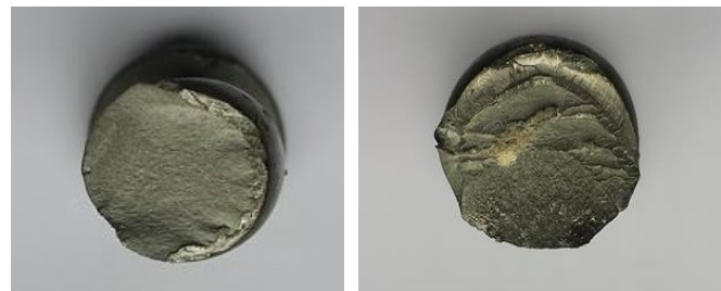
Figure 20: Fracture surface of PO-NW (left) and PL-1 (right)
