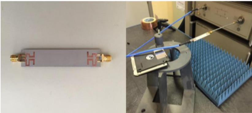
Fig. 2.15 Sample of waveguide and measurement setup
