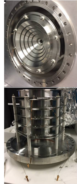
Figure 5: Left: technical drawing of the new setup. The gas cell (left volume) hosts from left to right the entrance window (blue), the cage (red), the funnel (green), the filament (cyan) and the nozzle (yellow). The gas jet chamber has a view port for the laser and a curved RFQ (purple) for ion extraction. For details see text. Right: Photographs of the funnel (top picture) and the cage structure (bottom picture) before installation.
