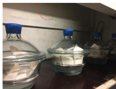
b. Samples in desiccators with salt solutions
