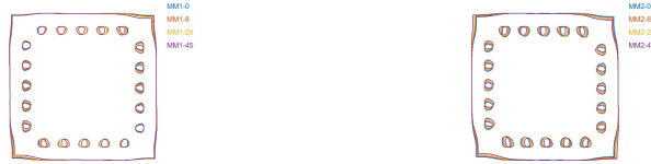
Figure 8: Deformed state of the different sample orientations tested in a PBR. It is not possible to estimate from the deformed state in a PBR whether the test axes and material axes are aligned.
