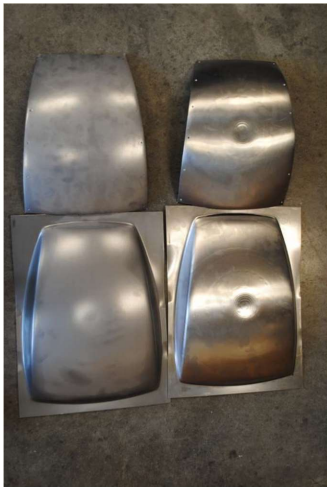
Fig. 7.10 HVAC shrouds manufactured by SPIF (Source: Department of Mechanical and Materials Engineering, Queen's University).
