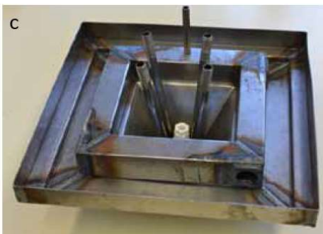
Fig 7.6 a) Cross section of four layered sheet die with integrated heating/cooling chambers for Resin Transfer Moulding (RTM) (1) sealing1, (2) high vacuum chamber, (3) sealing2, (4) RTM cavity, (5) Resin injection nipple, (6) RTM vacuum nipple, (7) water outlet upper die, (8) water outlet lower die, (9) high vacuum nipple, (10) & (11) water inlet lower and upper die. b) & c) Lower and upper die. (Source Mechanical Engineering department, KU Leuven)
