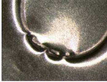
Fig. 3.3 A sample buckled part in micro-SPIF (Beltran, Malhotra et al. 2013).
