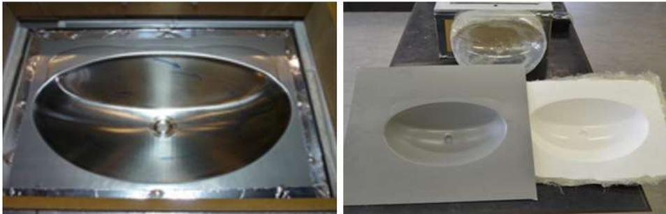
Fig 7.5 Stainless sheet die for a washbasin based on a perforated SPIF shell and low pressure moulding parts (hand lamination, RTM, thermoforming) (Source Mechanical Engineering department, KU Leuven)
