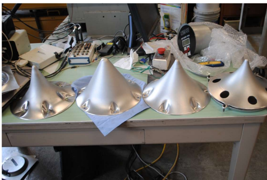
Fig. 7.8 Four examples of rapid prototypes for testing in an HVAC system (Source: Department of Mechanical and Materials Engineering, Queen's University).
