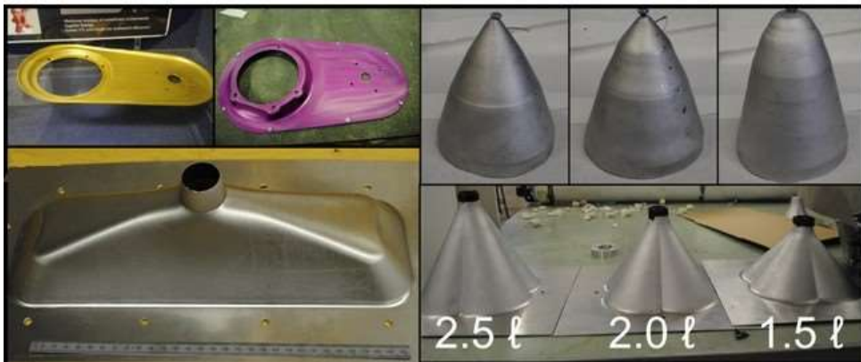
Fig. 7.7 Clockwise from top left: Automotive powertrain guards, diffuser cones for a gas turbine diffuser, engine air intake plenums for a race team, a different plenum design (Adams and Jeswiet, 2014b)
