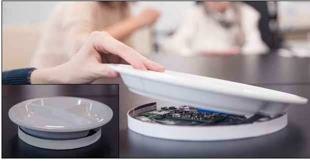
Fig. 1: The smart plate system: base station and plate.
