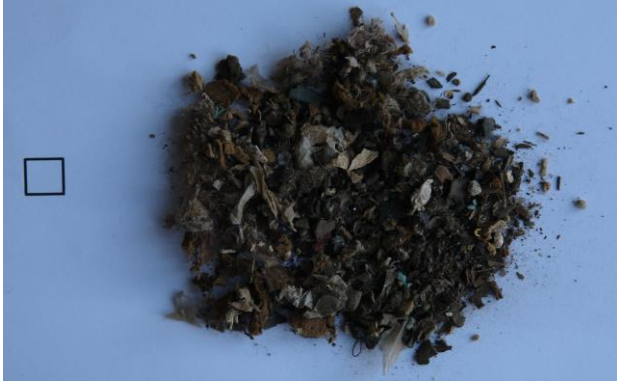
Figure 3: Photograph of the incinerated ASR (the real size of the black square is 10x10 mm)
