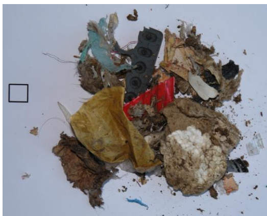
Figure 2: Photograph of the incinerated RDF (the real size of the black square is 10x10 mm)
