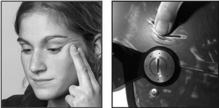
Figure 3-24: Illustration of natural protection of the head by the skin (left) and the stretchable low friction layer in SuperSkin helmet (right). From [98].
