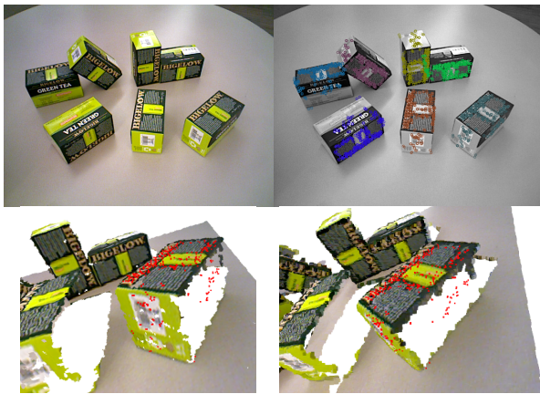
Figure 1: Given a single RGB-D image containing multiple instances of the same object (top-left), our method automatically discovers the object and localizes the multiple instances by grouping a set of features (top-right). A 3D model of the object is also recovered by registering the features from the multiple instances into a single coordinate system (bottom). The registered features are denoted as red dots, overlaid on the colored 3D point cloud of the scene. Note that some of the features appear on the missing face of this specific object instance, indicating that they are recovered from some other object instances.
