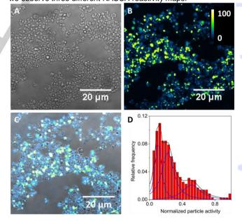
**Figure 2.** Transmission image (A) and 3D projection of a Z-stack (B) of 10 confocal images (0-10  $\mu$ m/0.25 $\mu$ m) of ZSM-5-507 zeolites after FFA reaction. The color scale indicates the normalized intensity. The correlated image of A and B (C) and a histogram of the normalized particle activity (D). The blue lines represent the Lorentzian fits, the black line is the sum of the three Lorentzians.
