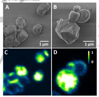
Figure 3. A) and B) SEM images of DAMPI-stained H-ZSM-5 crystals and C) and D) their respective confocal images.
