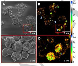
Figure 1. SEM image (A) and NASCA activity map (B) of H-ZSM-5 zeolites. C and D are enlargements of the areas indicated in A and B respectively. In B, the three types of crystals are indicated: 1: crystals with a homogeneous activity, 2: crystals where only the edge is active and 3: crystals that show almost no activity. The colour scale represents the normalized detected reaction rate per bin (50 x 50 nm<sup>2</sup>).
