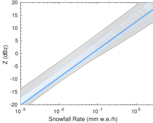
Figure 8: The 10<sup>th</sup> and 90<sup>th</sup> percentile uncertainty (blue shaded area) and the 1<sup>st</sup> and 99<sup>th</sup> percentile (grey shaded area) on the Ze-SR relation of all 12 snow storms with each 10,000 bootstrapping simulations. The ensemble average relation is denoted by the thick blue line.
