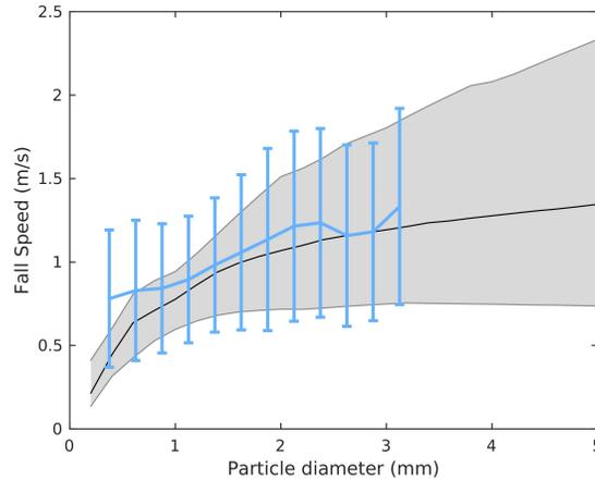
Figure 5: Median and 10<sup>th</sup> - 90<sup>th</sup> percentile terminal fall velocity calculated following the approach of Heymsfield and Westbrook (2010) (grey). The average of the direct measurements from the PIP (N=100,498) is shown including error bars showing 10<sup>th</sup> and 90<sup>th</sup> percentiles (blue).
