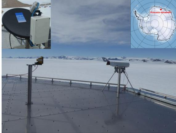
Figure 1: The PIP deployed on the roof of the Princess Elisabeth station. The camera is located in the heated housing on the right of the image, while the halogen lamp is on the left. The upper left inset shows the MRR, while the upper right inset shows the location of the Princess Elisabeth station.
