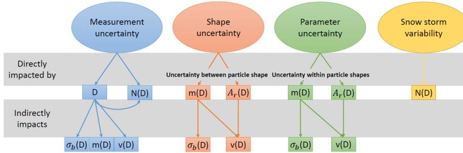
Figure 2: Overview scheme listing the four uncertainty terms and different terms contributing to each uncertainty. E.g. parameter uncertainty is directly impacted by the uncertainty of the mass of the particle for each particle shape and the area ratio, indirectly impacting the backscatter cross section and the terminal fall velocity of a snow particle, as uncertainties propagate into these parameters.
