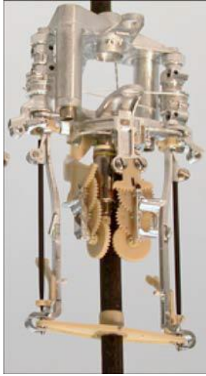
Fig. 9 The flapping mechanism of the Nano Hummingbird: A complex mechanism comprised of over 100 components.
