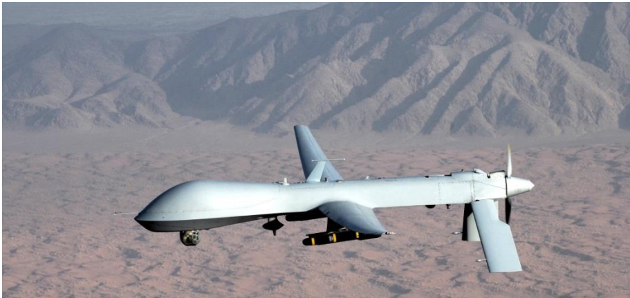
Fig. 2 Military drone, The RQ-1 PREDATOR with a wingspan of 16m [Predator, 2017]
