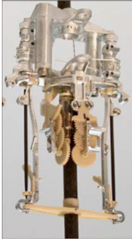
Fig. 62 Control mechanics of the Nano Hummingbird [Keennon et al, 2012] the two separate gear trains are responsible for reducing the motor speed of two actuators that control the variable wing twist modulation. The upper part of the mechanism controls the stroke motion.
