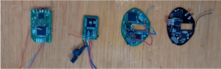
Fig. 72 The Control electronics of the Kulibrie: From left to right four consecutive versions of the control electronics of the Kulibrie.
