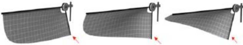
Fig. 61 Variable wing twist modulation: a flexible membrane is suspended between the leading edge and the root spar (red arrow). If the root spar rotates away from the wing, the thrust is increased. By rotating the root spar slightly around the leading edge a difference of angle of attack is realized between the forward and the back ward stroke. [Keennon et al, 2012]
