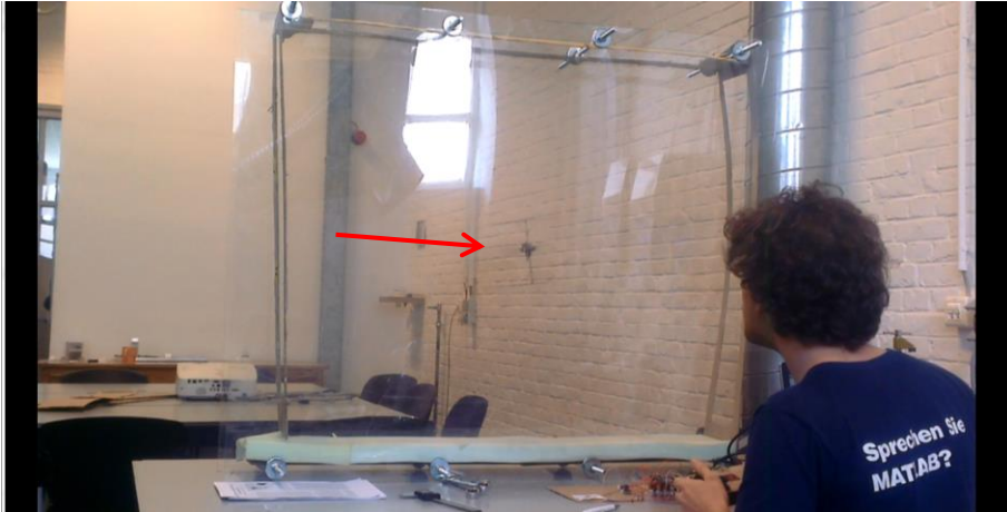
Fig. 83 Separately evaluating the active roll and pitch stabilization of the Kulibrie. The Kulibrie (indicated by a red arrow) flies between two transparent plates and is surrounded by a protective frame. The protective frame prohibits the wings from colliding with the plates and ensures that only a planar motion between the plates is possible.
