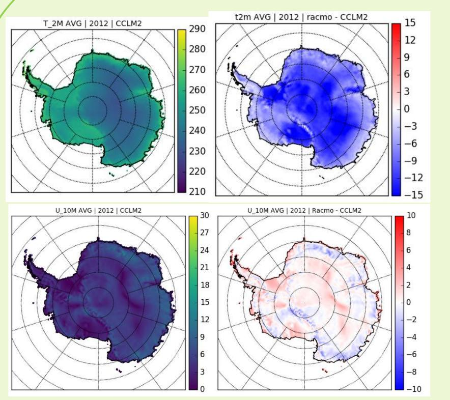
Figure 2: (left) Average temperature (up) and wind speed (down) for the year 2012. (right) Absolute difference with RACMO.
