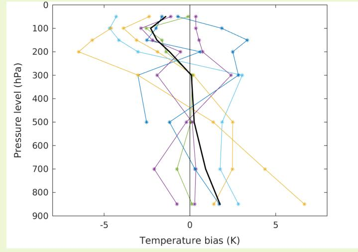
Figure 5: Temperature bias between balloon soundings averaged for January 2012 for eight stations (depicted by thin lines; figure 5) and the corresponding pixel in CCLM<sup>2</sup>. The average bias is depicted in black.
