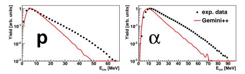
Fig. 2. Energy spectra of protons and  $\alpha$  particles emitted between 7° and 17° in the F-E channel of the reaction  ${}^{32}\text{S}{+}^{48}\text{Ca}$  at 17.7 MeV/*u* (experiment "III").
