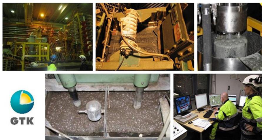
Fig. 3. Kvanefjeld ore froth flotation beneficiation pilot in GTK, Finland
