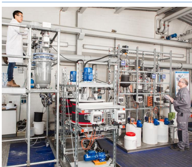
Fig. 4. Treatment of eudialyte concentrate was performed in the demonstration pilot plant at the IME Process Metallurgy and Metal Recycling laboratory of RWTH Aachen, Germany
