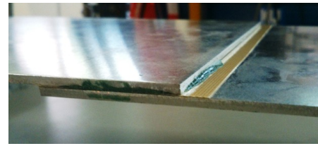
Figure 5. Adhesive bonding, with Teflon tape residue
