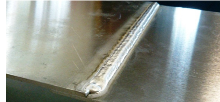
Figure 6. MIG weld connection
