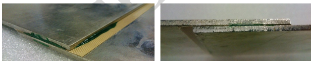
Figure 17. Excess glue and Teflon tape residue influence on width and thickness of bonding for adhesive bonded plates
