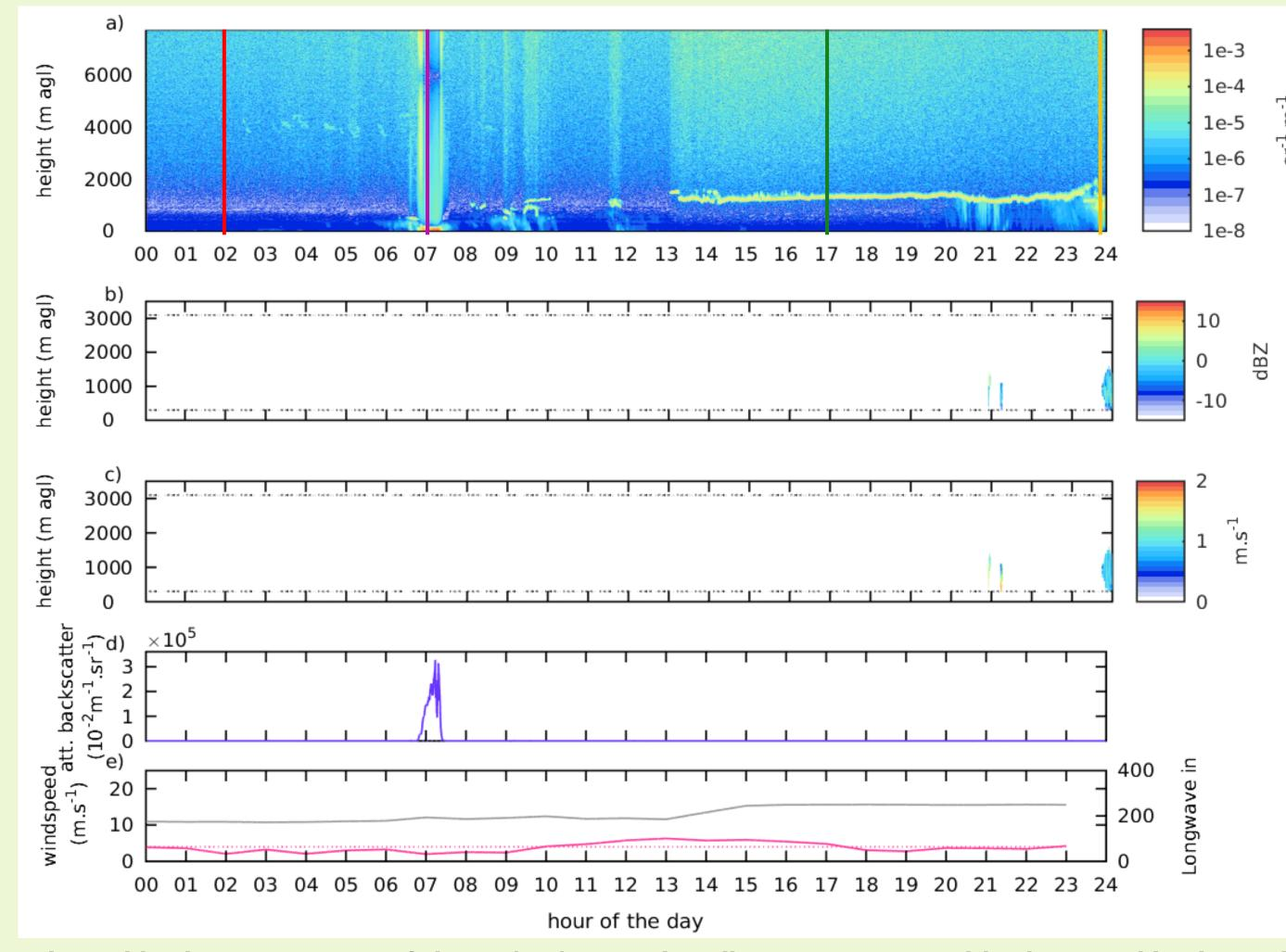
Fig. 5: blowing snow event of the 25/12/2013, a) ceilometer attenuated backscatter b) micro-rain radar effective reflectivity (in dBZ) c) Micro-rain radar Doppler velocity (in m s<sup>-1</sup>) d) ceilometer attenuated backscatter intensity at the ground level (in 10<sup>-5</sup> km<sup>-1</sup> sr<sup>-1</sup>) d) wind speed (pink, in m s<sup>-1</sup>) and incoming longwave radidation (grey, in W m<sup>-2</sup>) from the automatic weather station,
