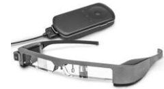
Epson Moverio BT-300 \mu display 1280x720 px
