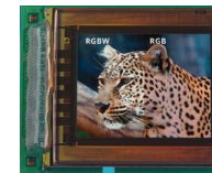
MicroOLED SXGA RGBW μdisplay 2687 ppi
