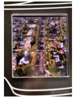
Sharp prototype panel 1008 ppi
